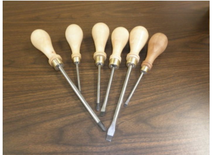
Screw Drivers with Turned Handles Hophornbeam wood known as Ironwood
