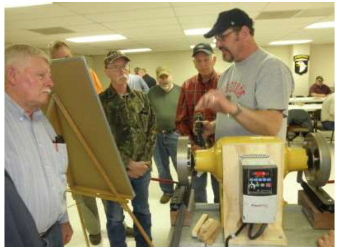
Steve explaining how to set up the Wolverine Sharpening Jig as members observe.
