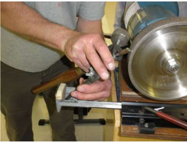
Steve shows how to sharpen a bowl gouge
