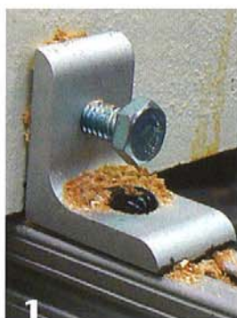
Arms on the frame have angle brackets that hold the shield in place against the lathe bed.
