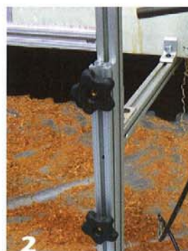
Vertical support legs can be adjusted for height.
