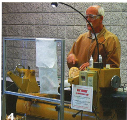
Jerry Kermode draped paper towels across the shield to protect it from splashes of finish.
