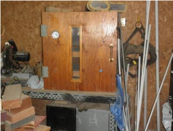
Incubator used for drying wood used in turning.
