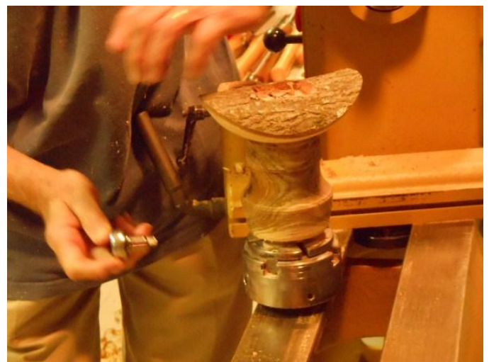
Jim trying to mount turned item into his 4-jaw chuck
