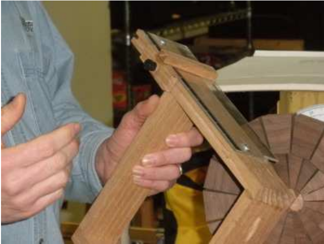
Kevin's home made jig for laying and gluing up the segments on the lathe.
