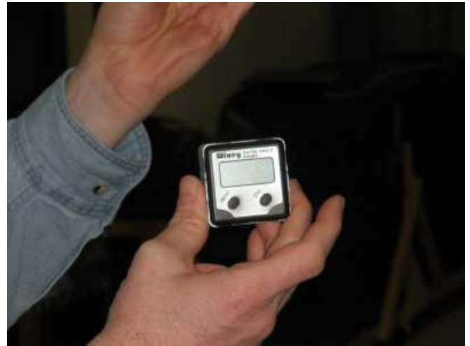
Kevin uses a wixey angle gauge to set the blade angle on his table saw, fence on his jointer, and table on his band saw, etc.
