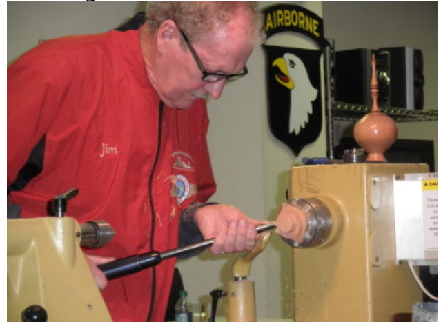
Jimmy demonstrates making the first part of a four part lidded box like the one pictured (top right).
