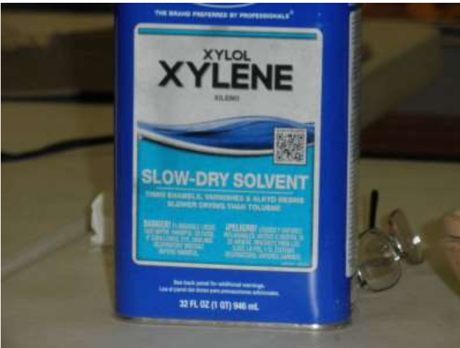
Xylene is used to transfer the image to the work piece.
