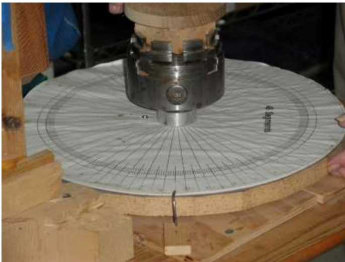
His indexing chart used for obtaining precise angles when cutting the hundreds of pieces in each of his turnings.
