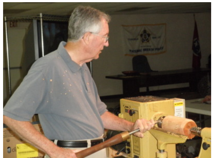
Jim Mason explains how to prepare the bottom for mounting either a face plate or a 4-jaw chuck by first mounting between centers.
