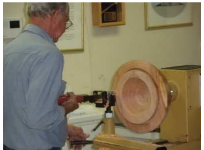
Here, Max is in the process of coring the second bowl. The first bowl has been removed.
